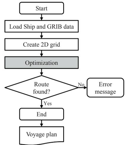
Fig. 3. Approach of the Vindskip™ Weather Routing Module
