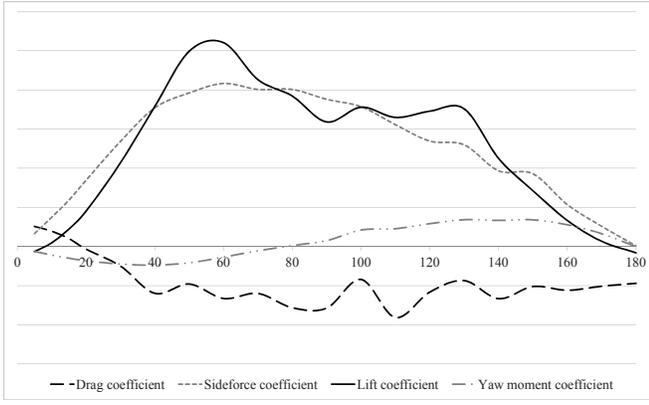
Fig. 6. Aerodynamic forces and moments of Vindskip™
