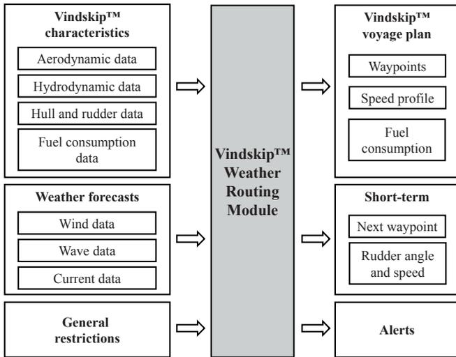
Fig. 2. Scope of the Vindskip™ Weather Routing Module
